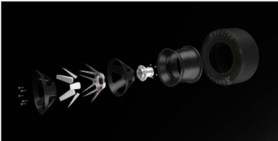
*Exploded assembly drawing of the wheel components*
