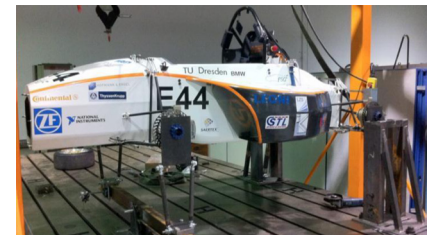
Monocoque on the torsion test bench.
